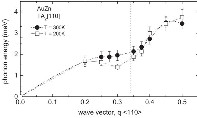
FIG. 3. Temperature dependence of the phonon dispersion in AuZn along the  $TA_2$  branch. At 300 K one notices considerable phonon softening at  $q = (0.33, 0.33, 0)$  (vertical line). The dashed lines between points are provided as guides to the eye.
