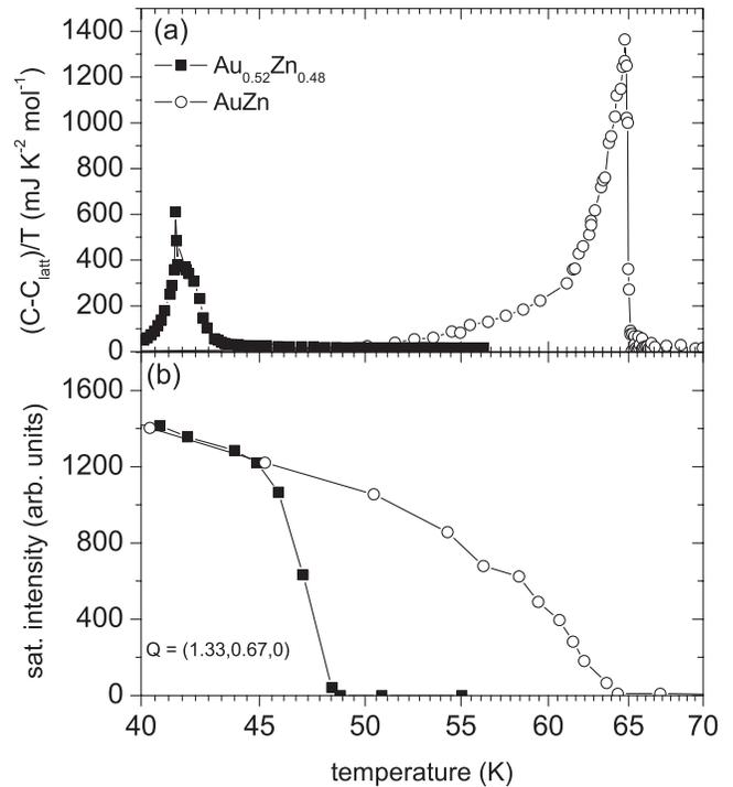
FIG. 1. (a) The excess specific heat divided by temperature versus temperature in the vicinity of the martensitic transitions for  $\text{Au}_{0.52}\text{Zn}_{0.48}$  and AuZn. (b) Temperature dependence of the satellite-peak intensity along  $Q = (1.33, 0.67, 0)$ . The satellite-peak intensity is proportional to the square of the order parameter.
